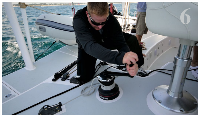
5- The Class 4's innovative solution for the mainsail halyard and reefing lines: a mini deck built around an electric winch integral to the mast. Just perfect!
